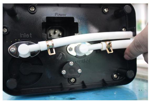
Fix another metal clip to the other piece of soft pipe, and connect it to the water outlet.
