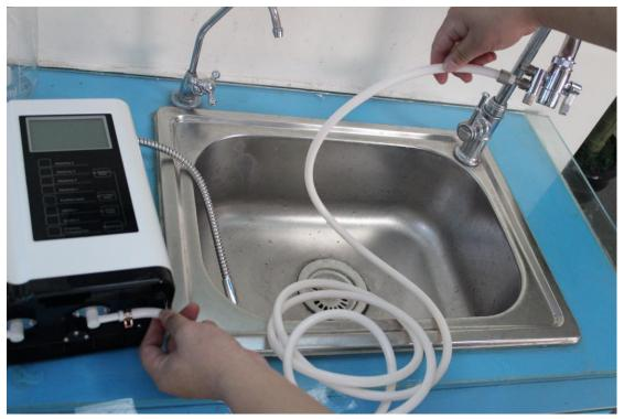
Connect another end of the pipe to the lower jack of the valve adaptor.
